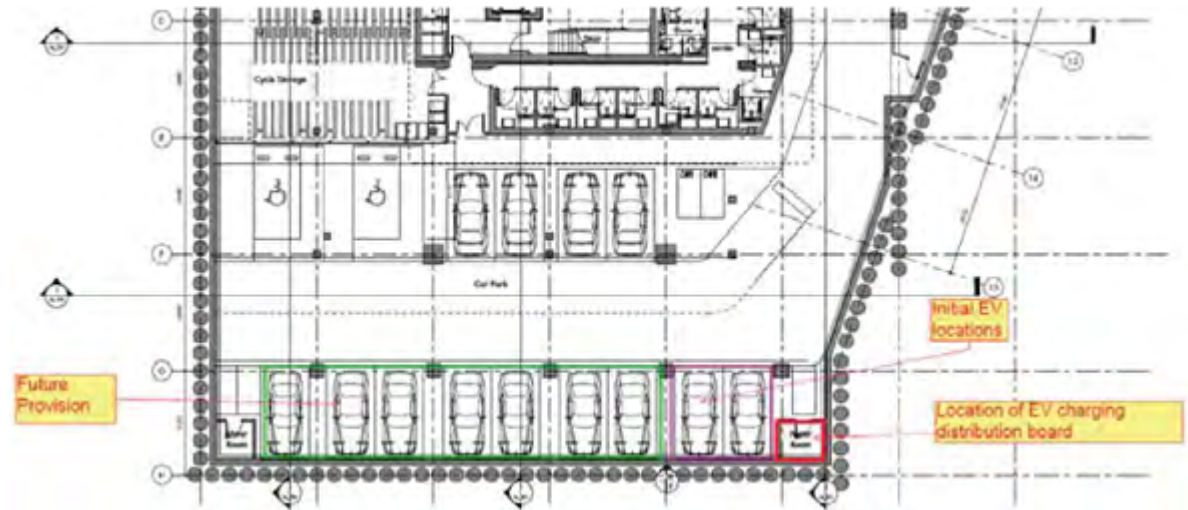
FIGURE 5.13 – EV CHARGING LOCATIONS & FUTURE PROVISION
