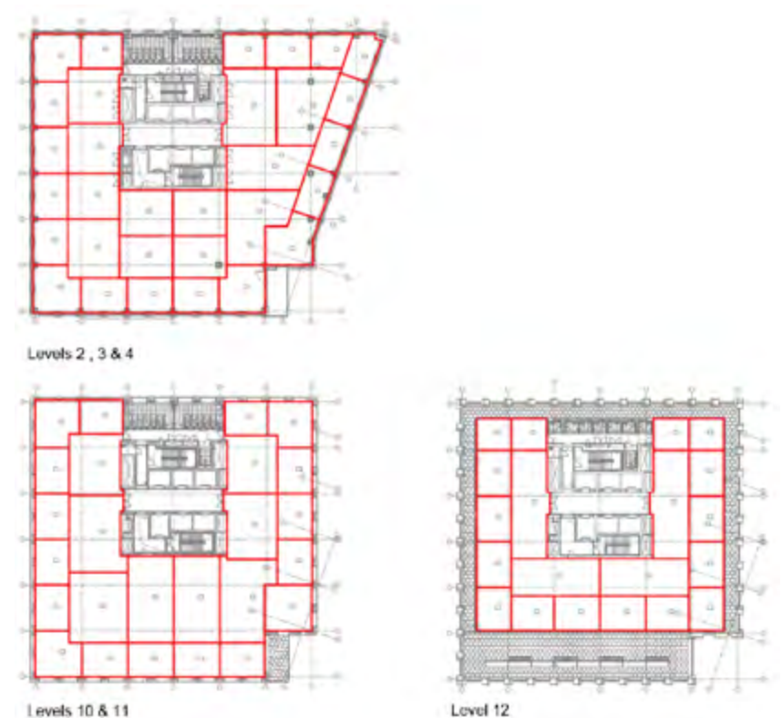
FIGURE 5.2 – TEMPERATURE CONTROL ZONES (CATEGORY A)
