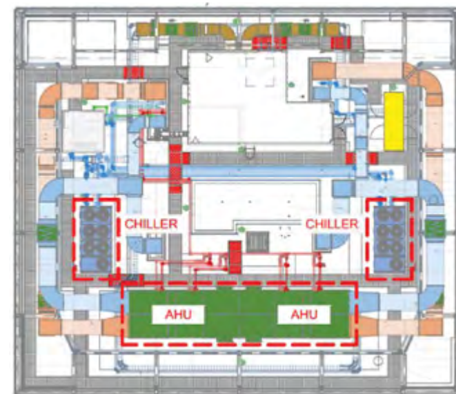
FIGURE 5.7 – AIR HANDLING UNITS AND CHILLERS AT ROOF LEVEL
