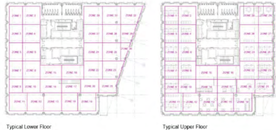
FIGURE 5.4 – LIGHTING CONTROL ZONES
